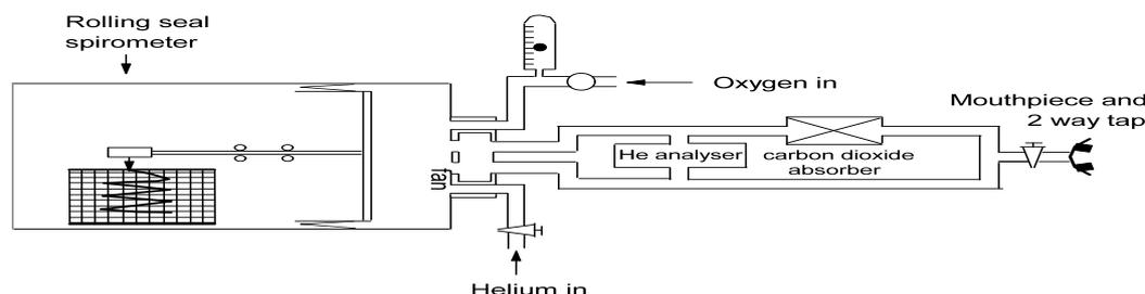
**Figure 7.2** Basic Components of a closed circuit system for measuring FRC by steady state He dilution technique.
