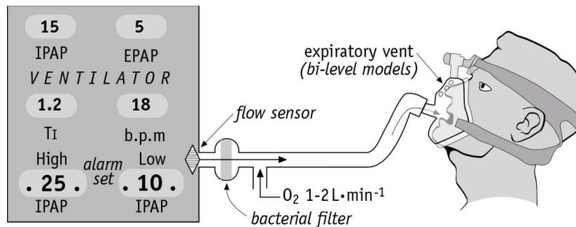
Figure 11.1 Diagram of ventilator circuit with bacterial filter, O<sub>2</sub> inflow, and 22 mm tubing attached to full face mask with in-built expiratory leak. Entraining oxygen nearer to the face mask gives a higher FIO<sub>2</sub>. Typical ventilator settings (cm H<sub>2</sub>O or s [TI]) shown for patient with neuromuscular weakness.
